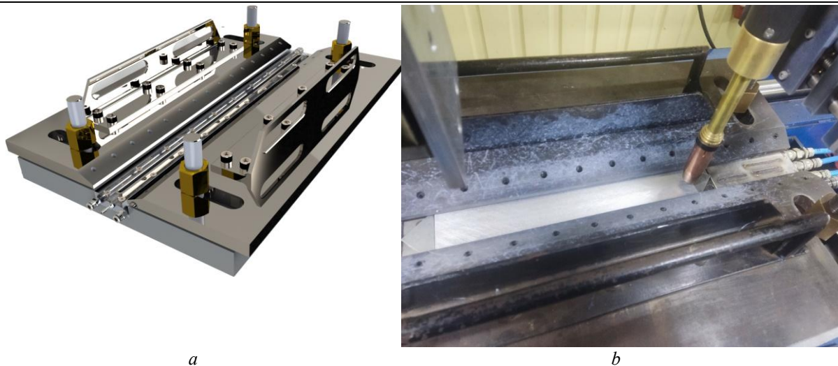
Figure 2. 3D model (a) and photograph of the assembly-welding fixture for butt joints (b)
