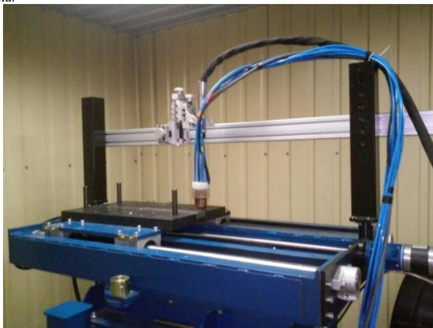
Figure 1. External view of the laboratory setup for MIG welding of butt joints of the 1561 alloy
